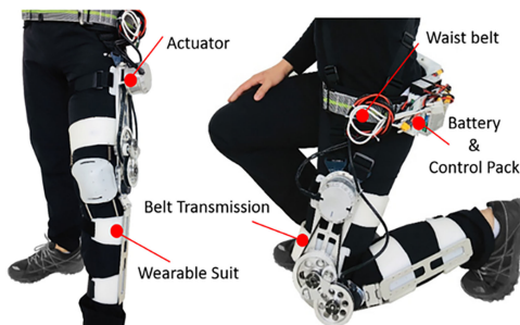
Fig. 1. A user wears the lightweight, compact and backdrivable knee exoskeleton in standing and kneeling postures, demonstrating its range of motion and compliance with human motion.
